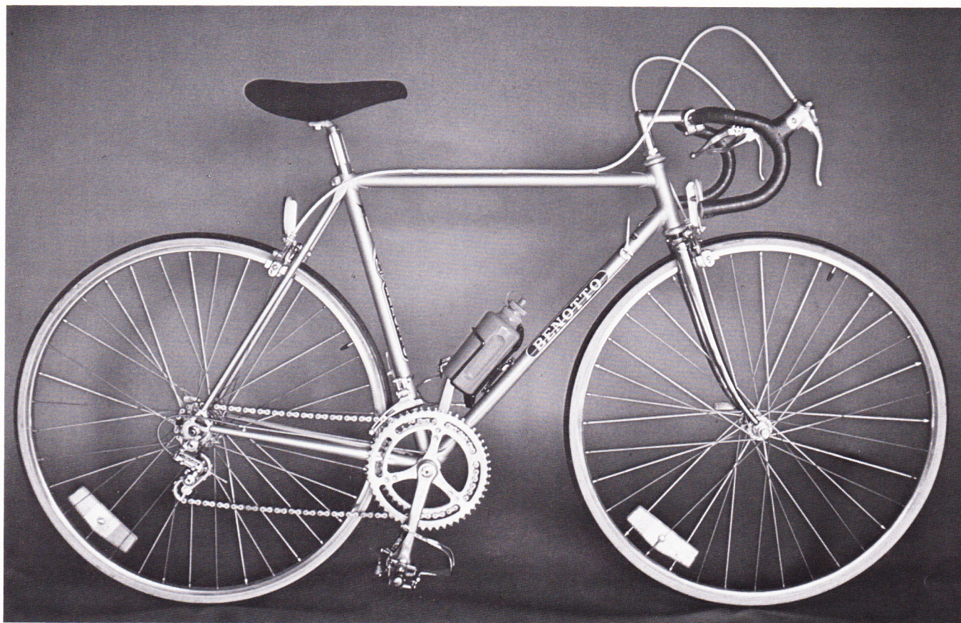
Bicycle with Benotto 2000 frameset and OMAS headset and OMAS titanium bottom bracket set weighing 19 lbs.
